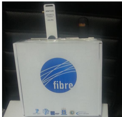
Figure 1 - Mini-itx based nodes, which are diskless nodes developed in the context of WP5 in order to increase the number of wireless devices.
